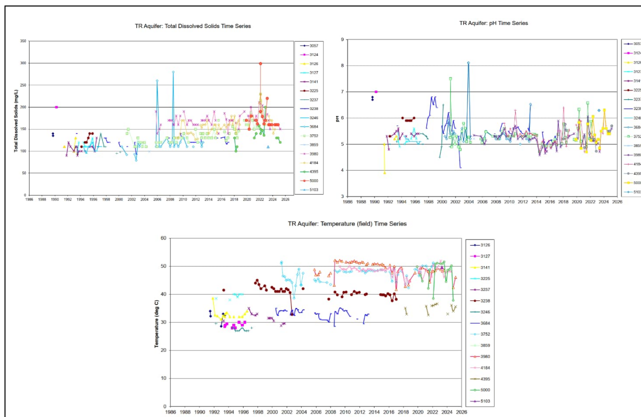
Figure 4-8 Historical time series for TR aquifer, TDS (top left), pH (top right) and temperature (bottom)
