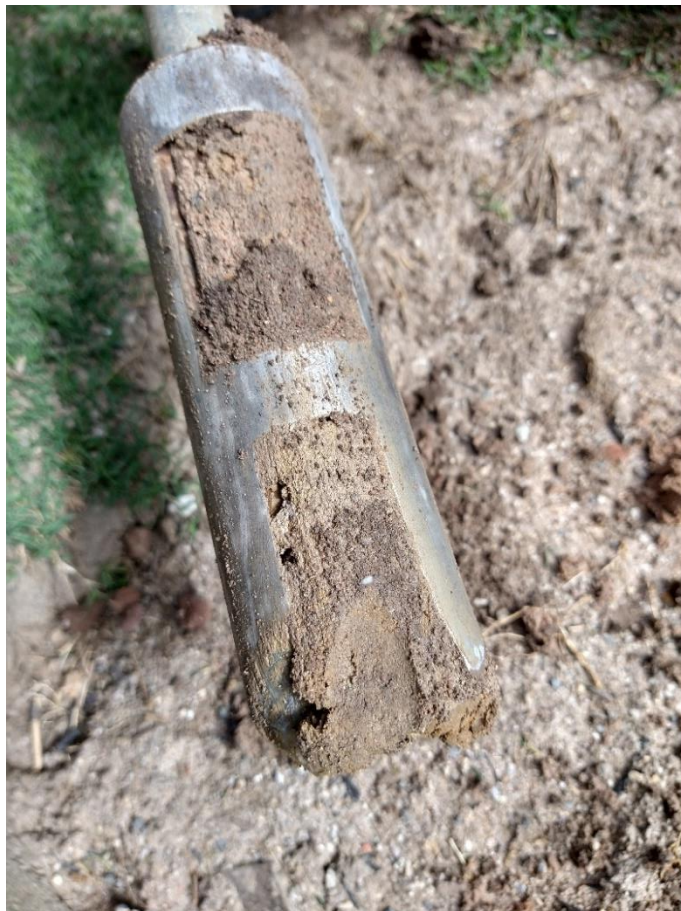
Photograph 1: Silty Sand and Silty Clay Layer from HA02
