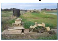
Most deliveries are through old inaccurate Dethridge wheels. These generally under-record deliveries to customers.
