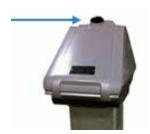
2. Unlock the controller housing lock on top of the gate's pedestal using the key issued with your manual.
